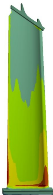
Figure 9 Normal stress field read in radial direction for a) nominal gas; and b) after fuel change.
