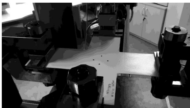
Figure 3 Biaxial testing machine with cross-shaped sample during test.
