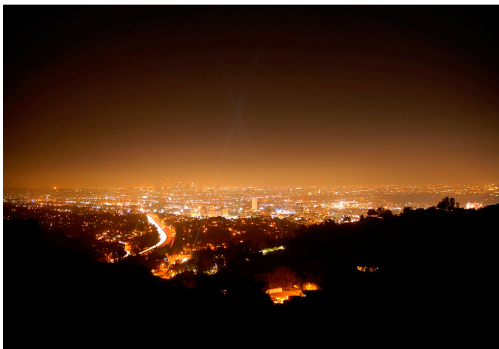
Figure 3. A typical city with a common problem: Man-made orange colored sky glow produced by high-pressure sodium light sources. Those cities that have retrofitted LEDs may have sky glow that is white in color. Source: Mike Knell/Flickr.
