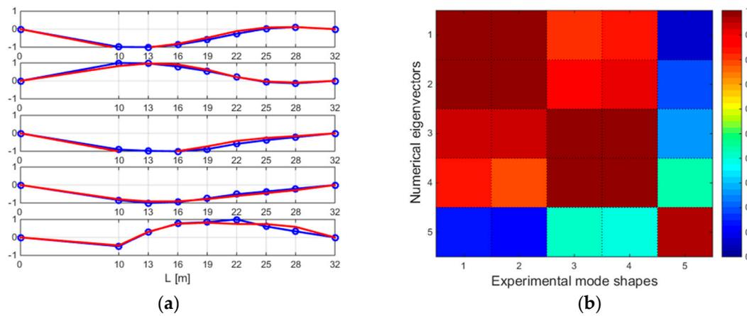
**Figure 17.** (a) Comparison of experimental vertical mode shapes (field test—blue; FEM model—red). (b) Representation of MAC matrix between the FEM model and filed test mode shapes of the arch bridge above the University Route in Bydgoszcz.
