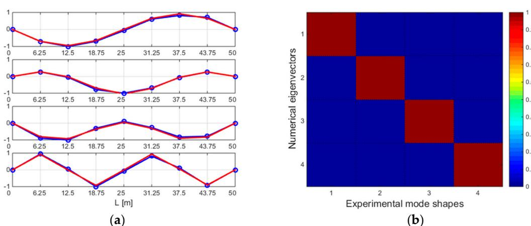
**Figure 16.** (a) Comparison of experimental vertical mode shapes (field test—blue; FEM model—red) (b) Representation of MAC matrix between the FEM model and filed test mode shapes of the arch bridge above expressway S8.
