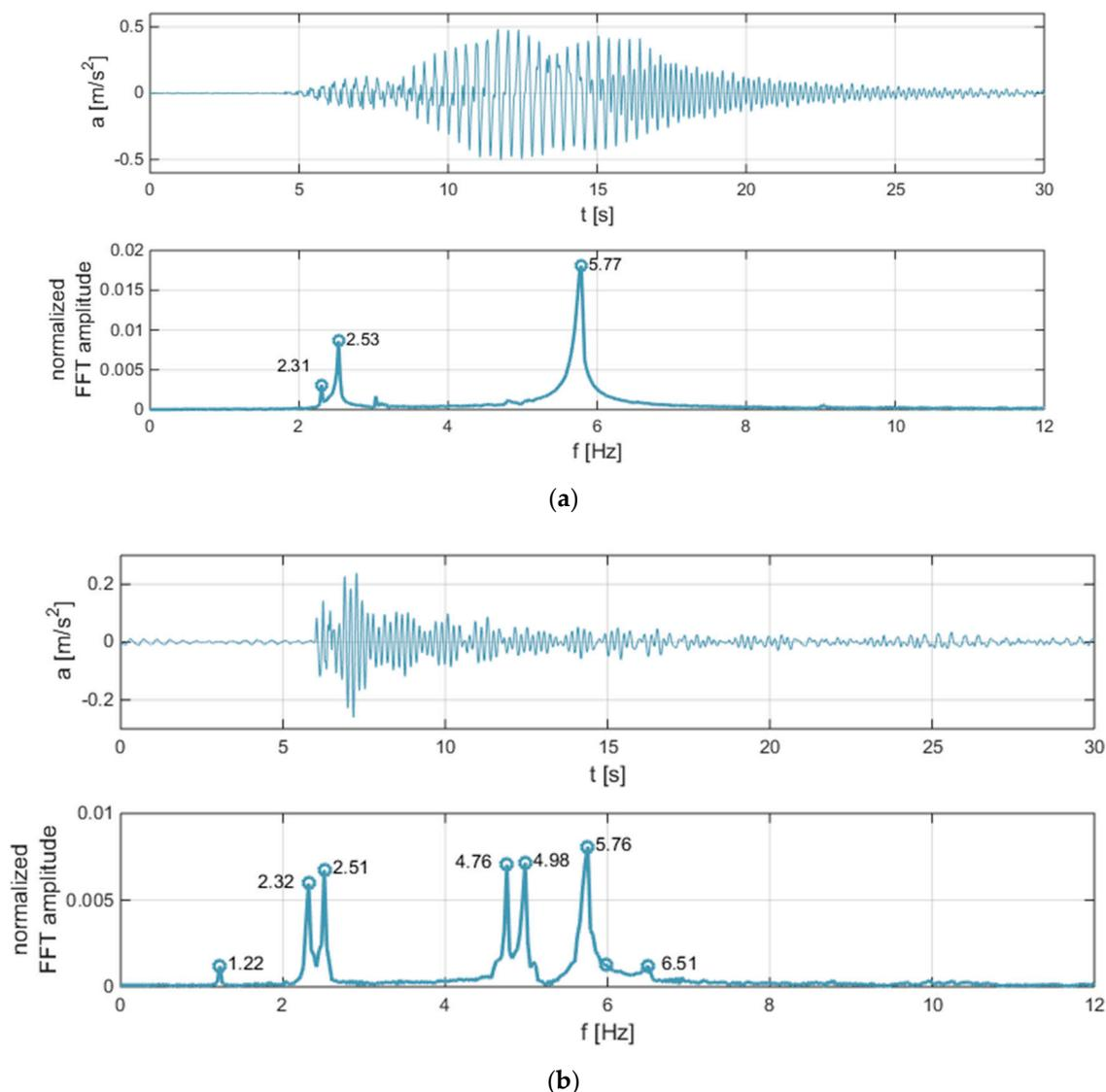
**Figure 10.** Time history of acceleration and normalized FFT amplitude for the arch footbridge above the University Route in Bydgoszcz at point a1z excited by (a) synchronous run of a group of nine persons, (b) impulse.
