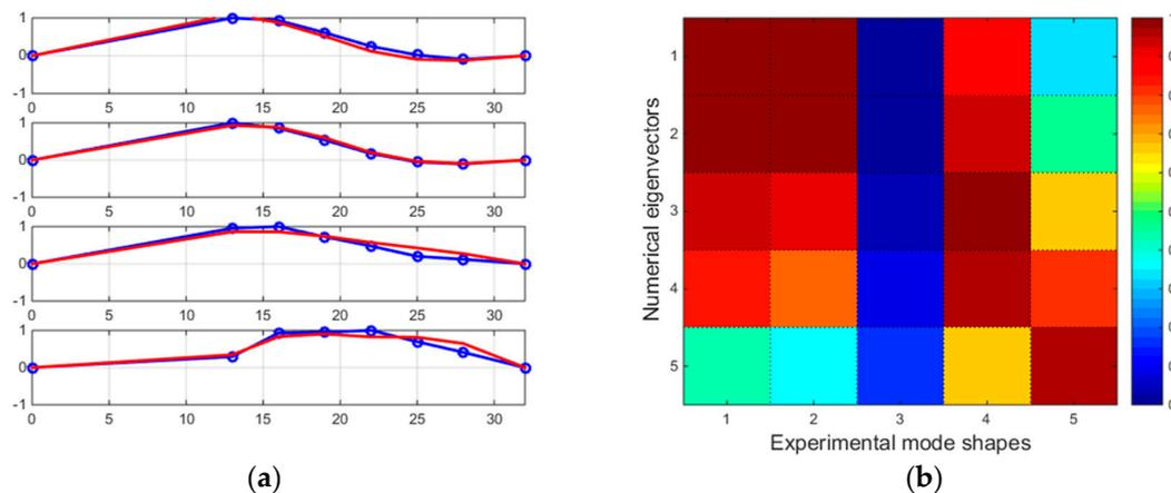
**Figure 18.** (a) Comparison of experimental vertical mode shapes (field test—blue; FEM model—red). (b) Representation of MAC matrix between the FEM model and filed test mode shapes of the arch footbridge above the University Route in Bydgoszcz.
