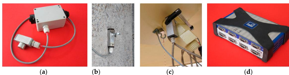
**Figure 5.** (a) Tri-axial MEMS accelerometer in a case; (b) Example of attaching the accelerometer on the concrete deck of footbridge; (c) Example of attaching the accelerometer on the elements of the hangers anchor of footbridge; (d) QUANTUM HBM 840a 8-channel measurement amplifier.
