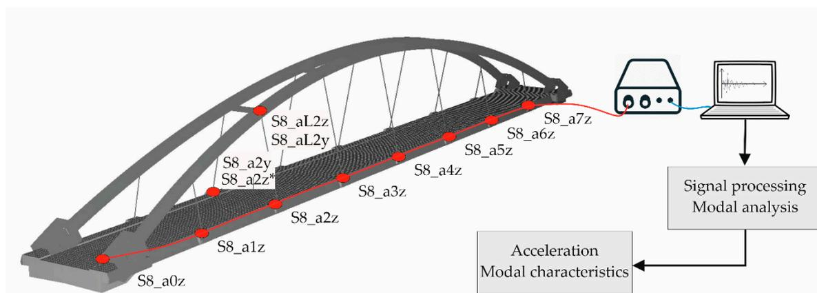
**Figure 7.** Dynamic measurement scheme of the arch footbridge above expressway S8.
