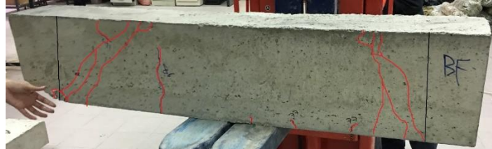
Fig.10: Beam (B2) at failure
