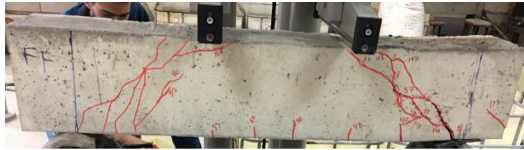
Fig.12: Beam (B4) at failure
