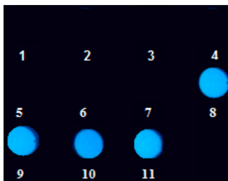
Figure 2. Photograph of oil drops of 11 samples applied to a black matte plate, placed in a dark place and illuminated with a UV LED lamp at \lambda = 365 nm. The sample type is presented in Table 1, please refer.
