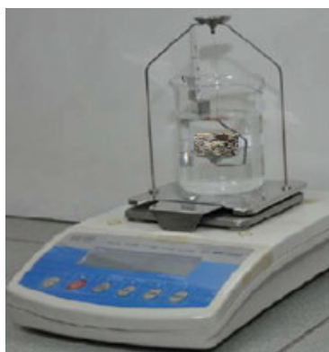
Figure 2. Density measurement by means of the hydrostatic method.
