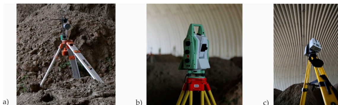
Figure 4. Devices and sensors used to measure basic bridge properties: (a) vertical translation inductive sensor, (b) total station, (c) laser scanner.
