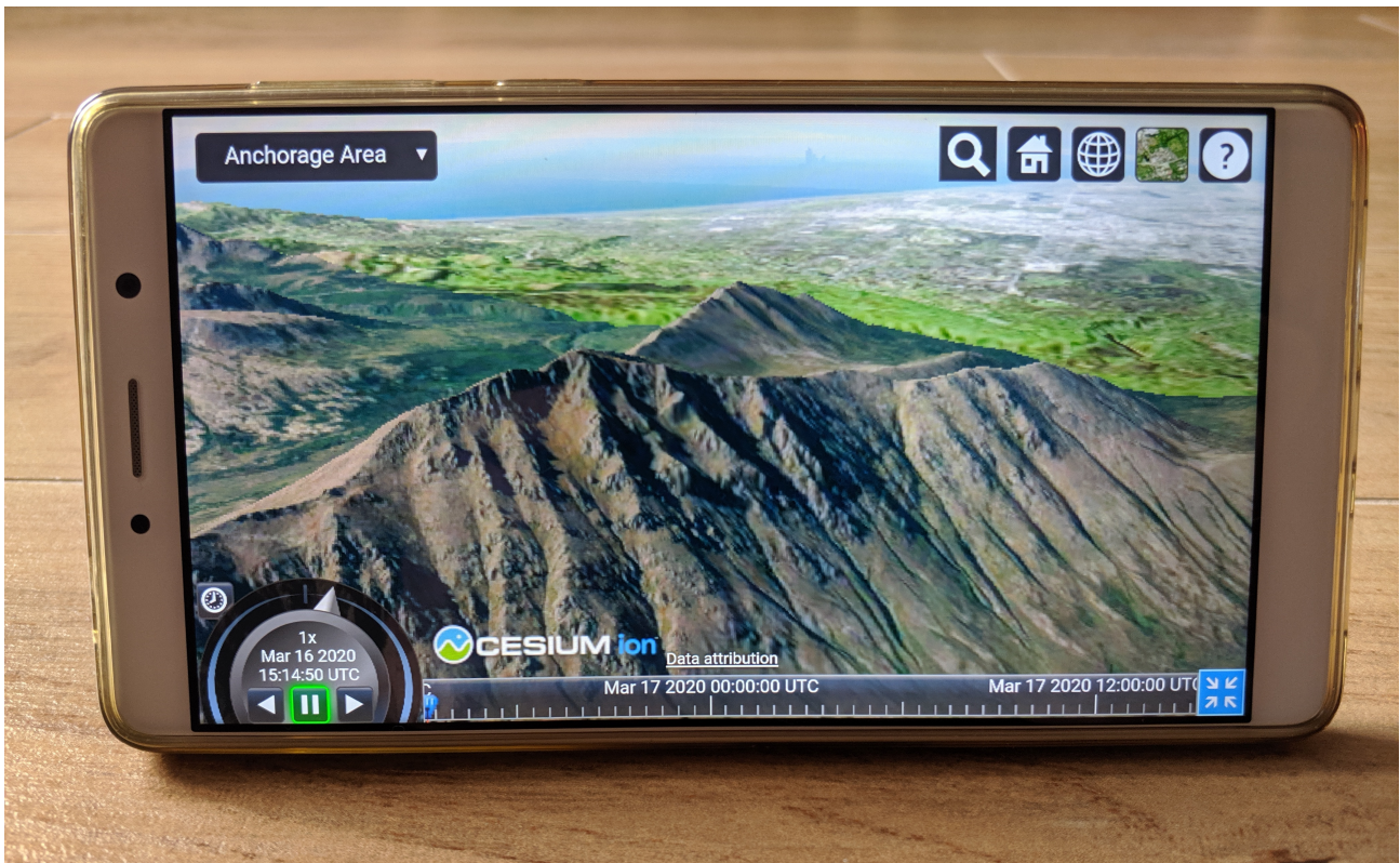
Figure 10. A mid-range smartphone produced in 2016 can provide smooth rendering of 3D terrain in a web application created using the Cesium library. Source: own study.
