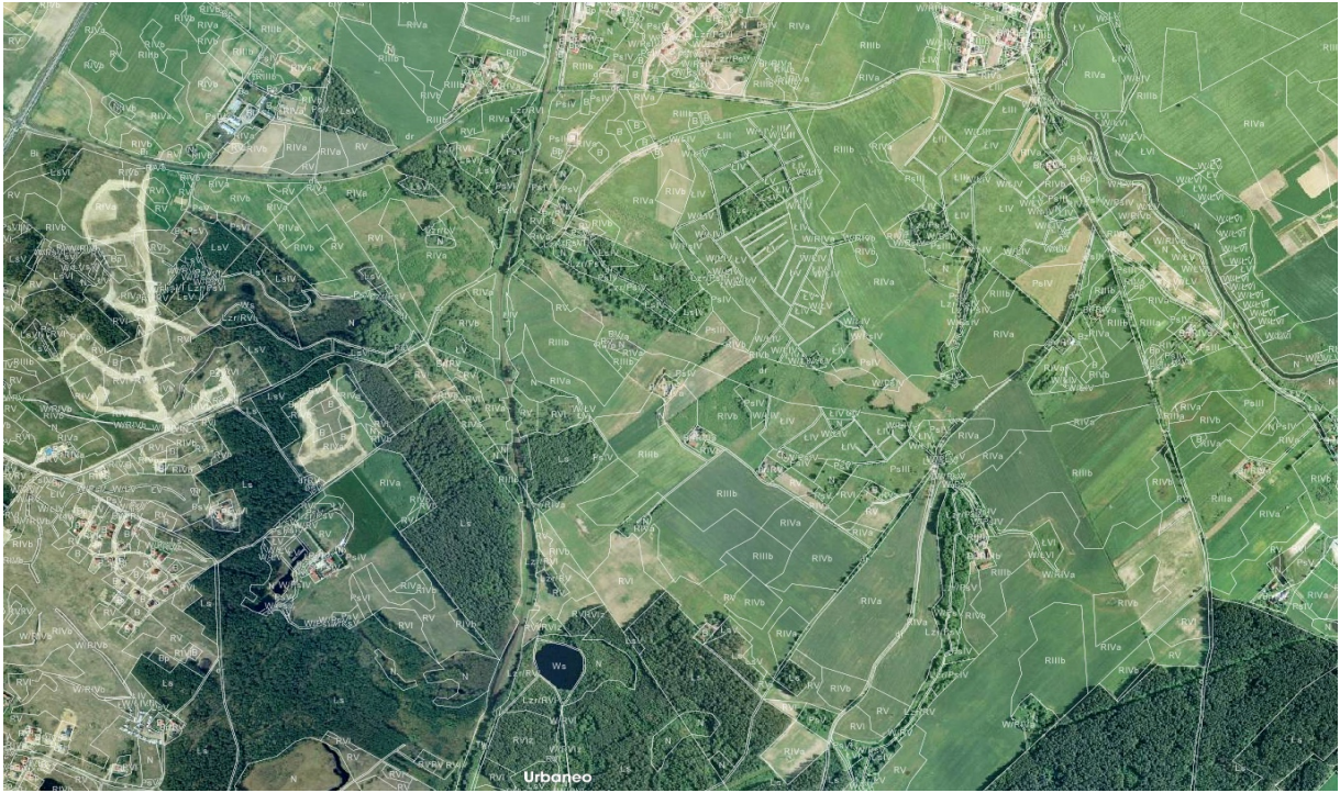
Figure 6. An image from the Land Information System of Stawiguda, Poland, depicting land use parcels overlaid on an orthophotomap of the area. Although the vector map shows an outline of a new road, the background map does not properly represent it.
