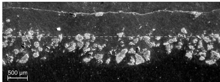
Figure 7. Cross-section through a composite layer based on Al6061 alloy with TiC powder; experimental conditions: I = 400 \text{ W/mm}^2 , v_{sc} = 10 \text{ mm/s} , m_p = 6 \text{ g/min} .
