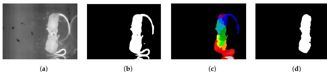
Figure 1. Results of the most popular algorithms used for segmentation of (a) original image by: (b) Otsu's thresholding, (c) watershed with gradient regions markers, (d) U-Net—semantic segmentation.
