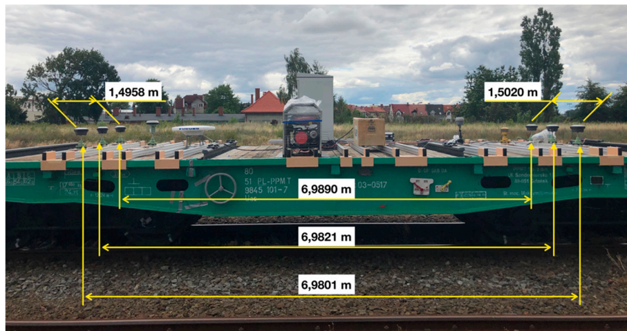
Figure 4. Determined distances between antennas on the surveying platform.
