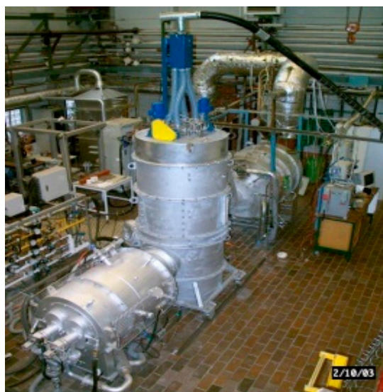
Figure 8. Experimental stand for continuous downdraft gasification.
