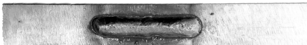
Figure 7. Macroscopic view of the bead-on-plate weld.
