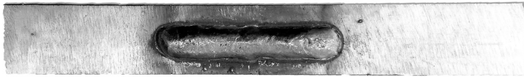
Figure 7. Macroscopic view of the bead-on-plate weld.
