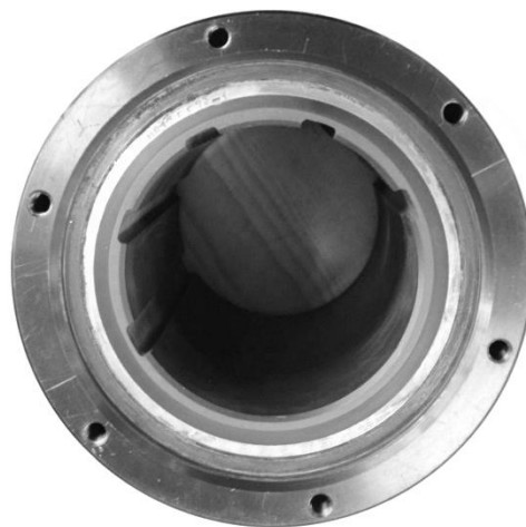
Fig. 2. Side view of the tested stern tube water-lubricated bearing assembled in the test-stand housing.
