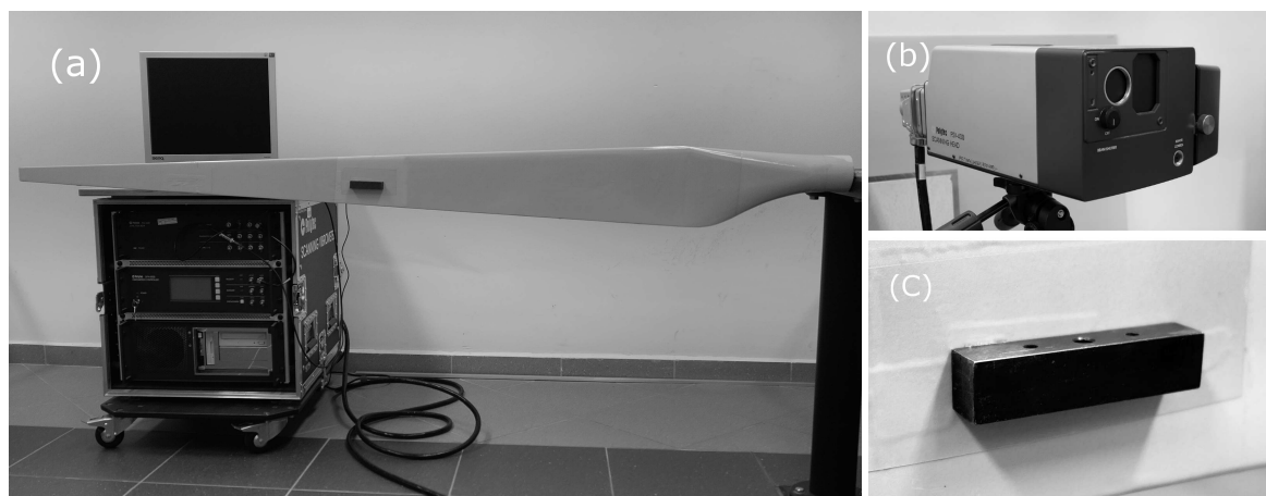
Figure 10. The experimental set up in laboratory: (a)—tested blade and equipment of LSV, (b)—head of laser scanning vibrometer, (c)—model of the damage.
