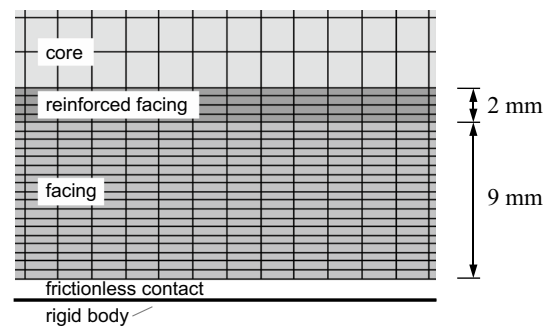
Fig. 5 FE mesh fragment with layer arrangement and a rigid body contact zone
