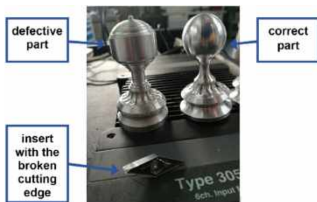
Fig. 2 Sample parts produced on a four-axis CNC ST20Y Haas lathe
