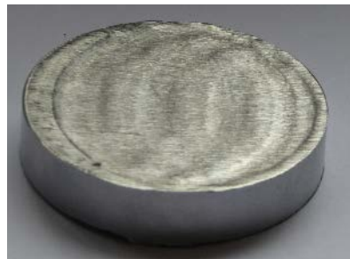
Figure 4. General view of the sample #1 with the washboard pattern on the sawn surface.
