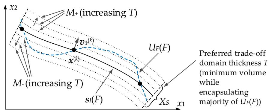
**Figure 3.** The meaning of the domain thickness parameter  $T$ , here, explained for two-dimensional parameter space. Increasing  $T$  enlarges the model domain which allows for encapsulating the optimum design manifold  $U_F(F)$ . At the same time, larger domain requires more training samples to render reliable surrogate. The desired trade-off is to find the minimum value of  $T$  enabling incorporation of the majority of  $U_F(F)$  into  $X_S$ .
