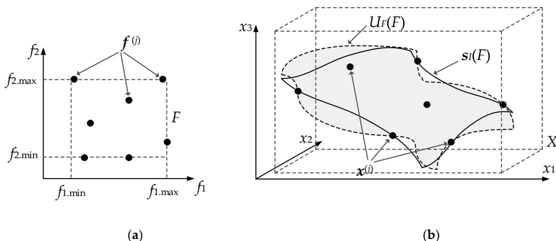
**Figure 1.** Fundamentals of the nested kriging concept (here, shown for two performance figures and three-dimensional parameter space): (a) objective space  $F$ , (b) parameter space  $X$ , the reference designs, the optimum design manifold  $U_F(F)$ , and the first-level model image  $s_I(F)$ . The manifolds  $U_F(F)$  and  $s_I(F)$  do not coincide for all  $f \in F$  but the agreement is perfect for all reference designs  $x^{(j)}$ , which are optimal in the sense of (1).
