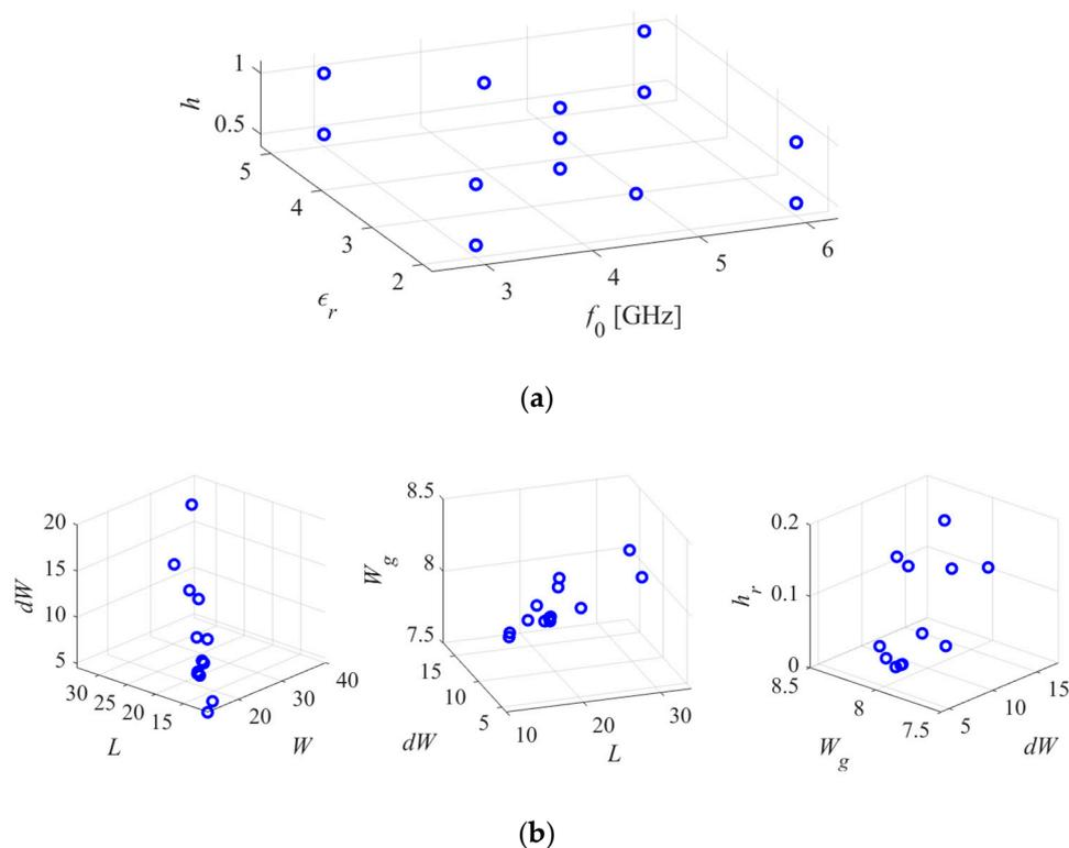
**Figure 12.** Allocation of the reference designs for the antenna of Figure 11: (a) objective space, (b) selected three-dimensional projections of the parameter space.
