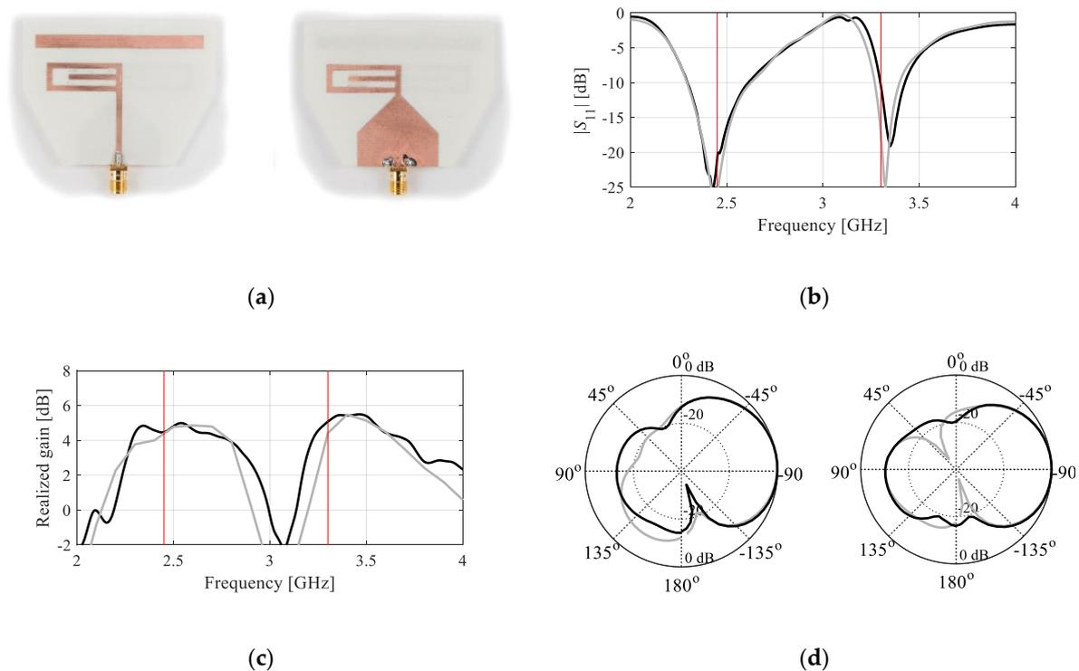
**Figure 10.** Antenna of Figure 6 optimized for  $f_1 = 2.45$  GHz,  $f_2 = 3.3$  GHz: (a) photographs of the prototype, (b) reflection  $|S_{11}|$ , (c) end-fire realized gain, (d)  $yz$ -plane radiation pattern at both operating frequencies (2.45 GHz and 3.3 GHz on the left- and right-hand-side, respectively). Simulated and measured characteristics shown in gray and black, respectively.
