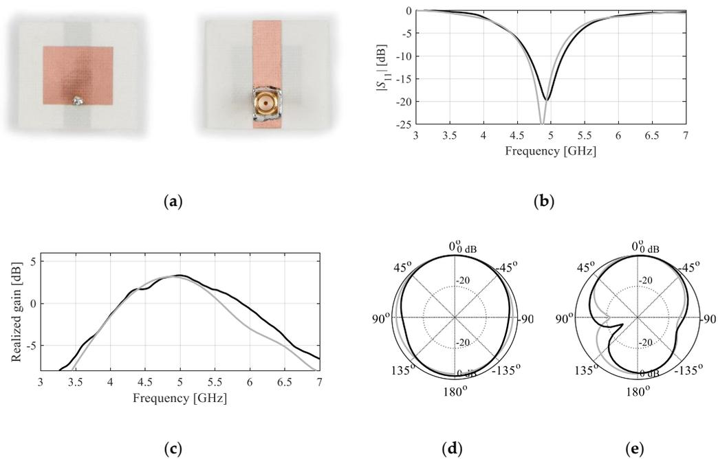
**Figure 15.** Antenna of Figure 11 optimized for  $f_0 = 4.8$  GHz,  $\epsilon_r = 3.38$  and  $h = 0.51$  mm, implemented on RO4003C substrate: (a) antenna prototype, (b) reflection, (c) realized gain, (d) H-plane pattern at 4.8 GHz, (e) E-plane pattern at 4.8 GHz; simulations (gray) and measurements (black).
