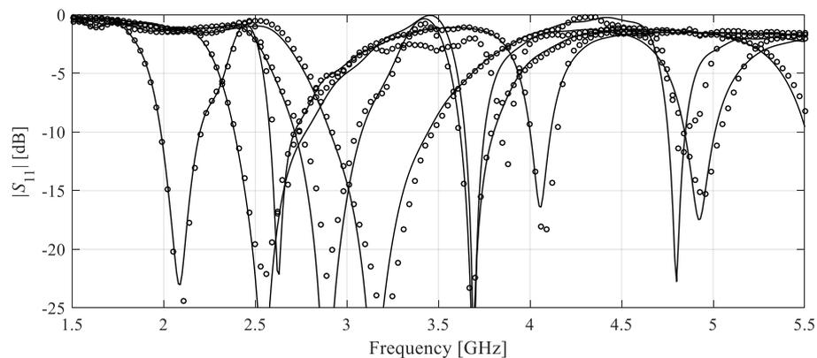
**Figure 8.** Dipole antenna: reflection responses at the selected test designs: EM model (—), nested kriging with variable-thickness domain obtained using 400 training samples and  $T_{\max} = 0.02$  (o).
