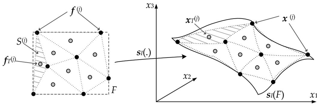
**Figure 4.** Triangulation of the reference designs performed in the objective space. The centers  $f_T^{(i)}$  of the resulting simplices  $S^{(i)}$  are mapped into the parameter space as  $x_T^{(i)} = s_i(f_T^{(i)})$ .
