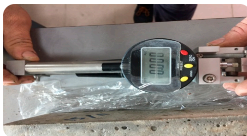
Figure 7. Mechanical strain gauge.
