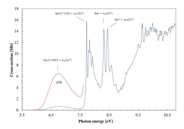
Fig. 2. An enhanced plot for the VUV photoabsorption spectrum of CH<sub>3</sub>OH in the 7.5–9.2 eV photon energy range. See text for details.
