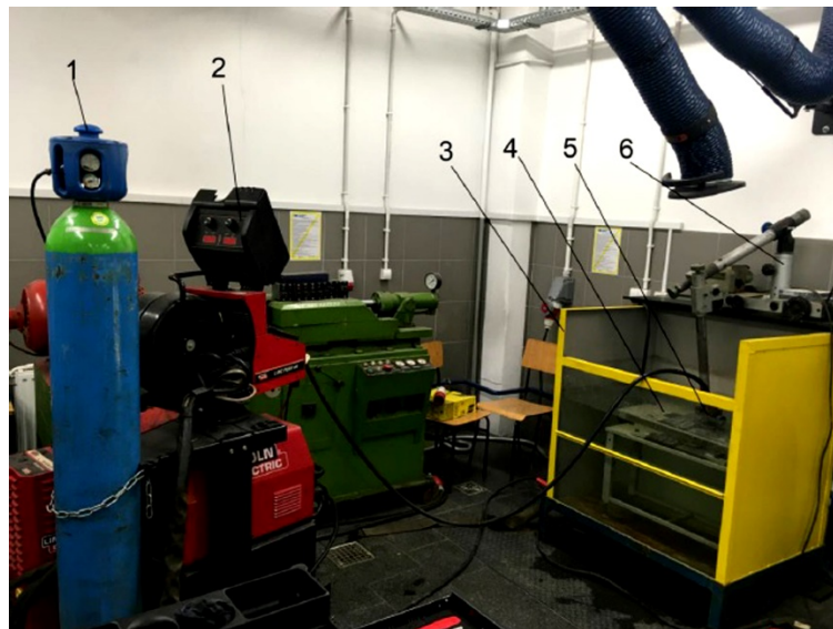
Figure 1. Welding test stand: 1-gas cylinder, 2-welding power source and wire feed unit, 3-tank, 4-welding table, 5-specimen, 6-welding trolley (tractor).
