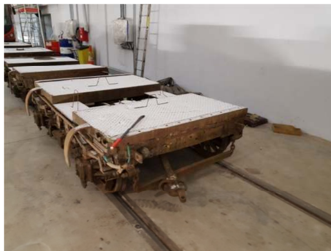
6. Bogies of a GWF 300 series wagon used as measuring vehicles
