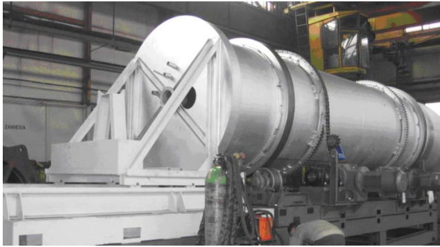
Fig. 3. Detailed view of the rotary pyrolysis chamber.
