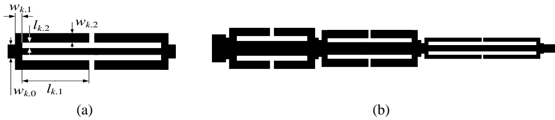
Fig. 4. Three-section 50-to-100 ohm impedance matching transformer: (a) basic building block of the transformer: compact microstrip resonant cell (CMRC) cell, (b) transformer geometry.
