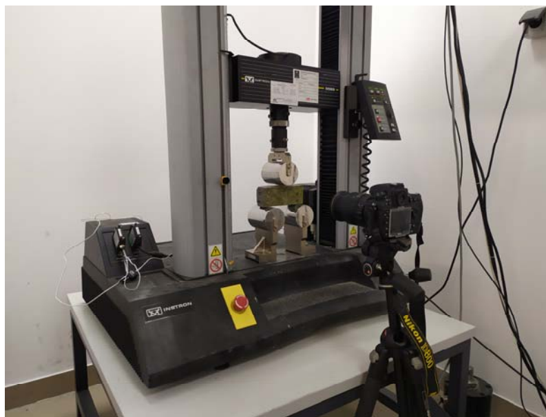
178 179 180 Figure 3: View on the DIC testing station. Digital NIKON D800 camera is mounted on a tripod 181 perpendicularly to the concrete beam placed in Instron 5569 static machine 182
