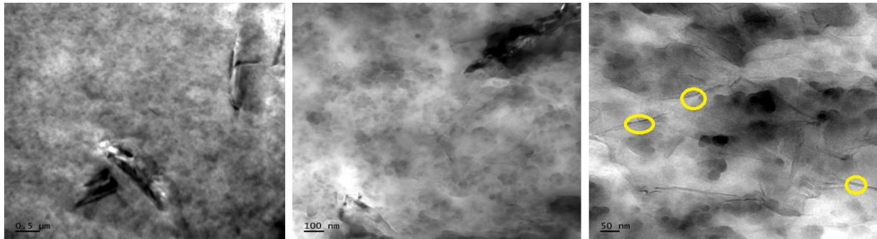
Figure 11. TEM images of QMEG7 composite and yellow circle indicate the layers of EG.
