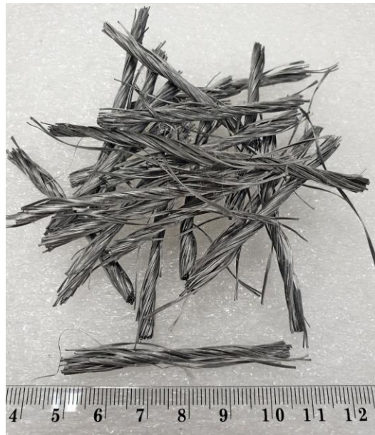
Figure 2. Photograph of twisted-bundle macro-polyolefin fibres
