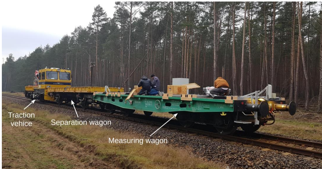
Fig. 8. View of the measuring train.
