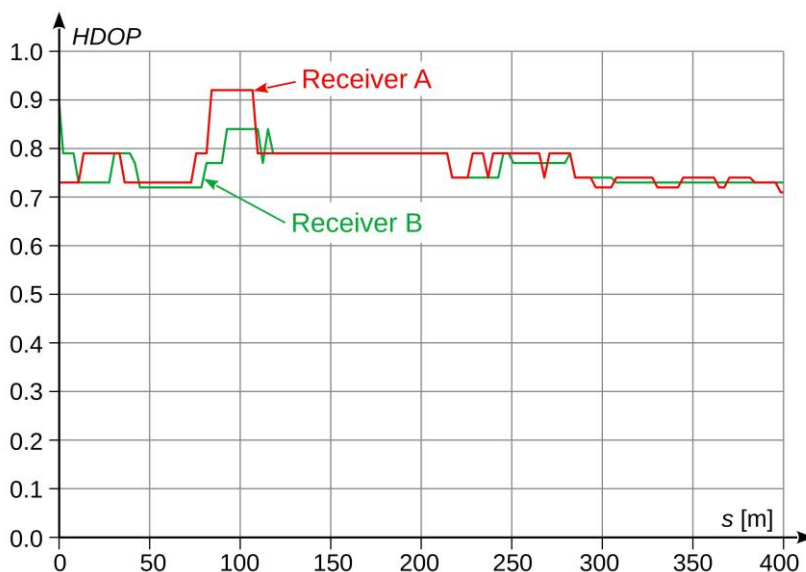
Fig. 21. Distribution of HDOP values along the test section
