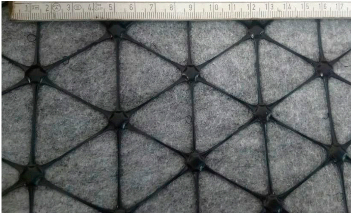
Figure 2. View of the AX5-GN composite, hexagonal geogrid bonded to non-woven geotextile.
