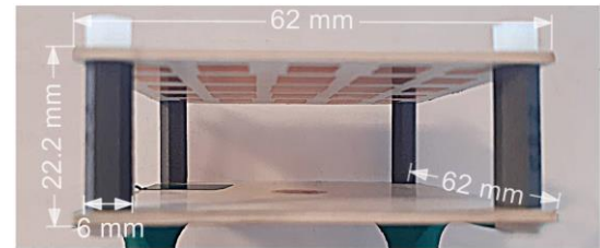
Fig. 6. Fabricated X-band antenna with the proposed superstrate layer.
