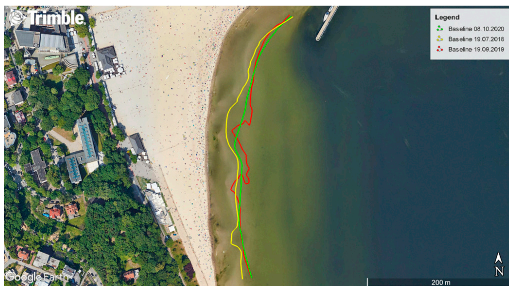
Figure 5. The course of the TSB of the waterbody adjacent to the public beach in Gdynia measured with the hydrographic method in 2018–2020.
