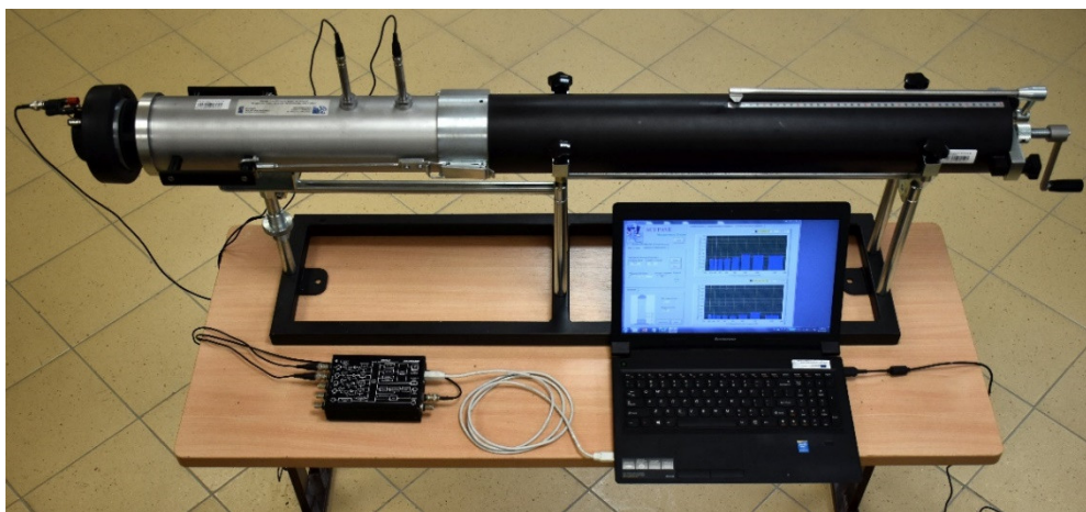
Figure 4. Spectronics ACUPAVE System measurement set.
