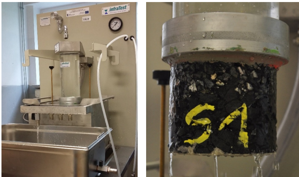
Figure 6. Vertical water permeability test.
