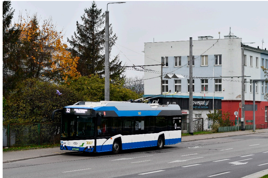
Figure 3. The process of automatic connection to the overhead line of a Solaris Trollino 12 M trolleybus on line 32 (photo taken by K. Grzonka).
