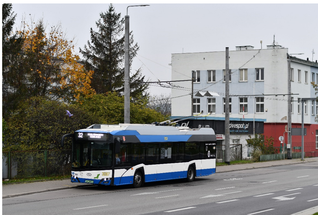
Figure 4. Automatic connection of an IMC trolleybus to the OHL (photo taken by K. Grzonka).
