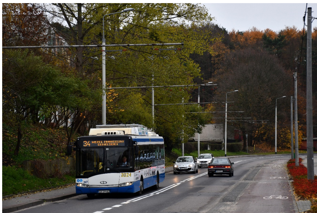
Figure 3. A trolleybus driving on battery power under the OHL due to the absence of an adequate site to connect the pantographs to the catenary (photo taken by K. Grzonka).
