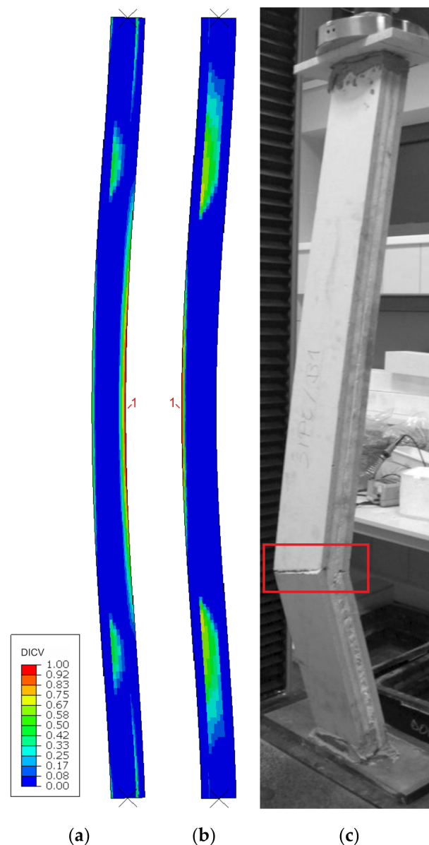
Figure 10. Comparison of failure modes in the L3 sample compression test obtained from FEA (a) MgO min, (b) MgO max variants, and (c) experimental observation.
