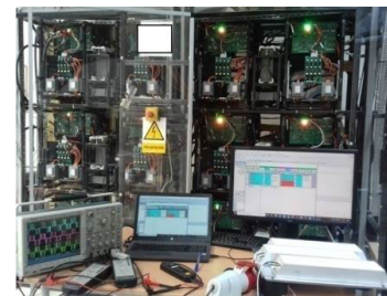
FIGURE 9. Laboratory prototype stand for the 7-level CHB MLI.
