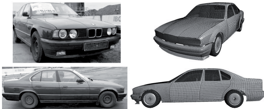
Fig. 4. Comparison between the full-scale BMW vehicle and corresponding numerical model
