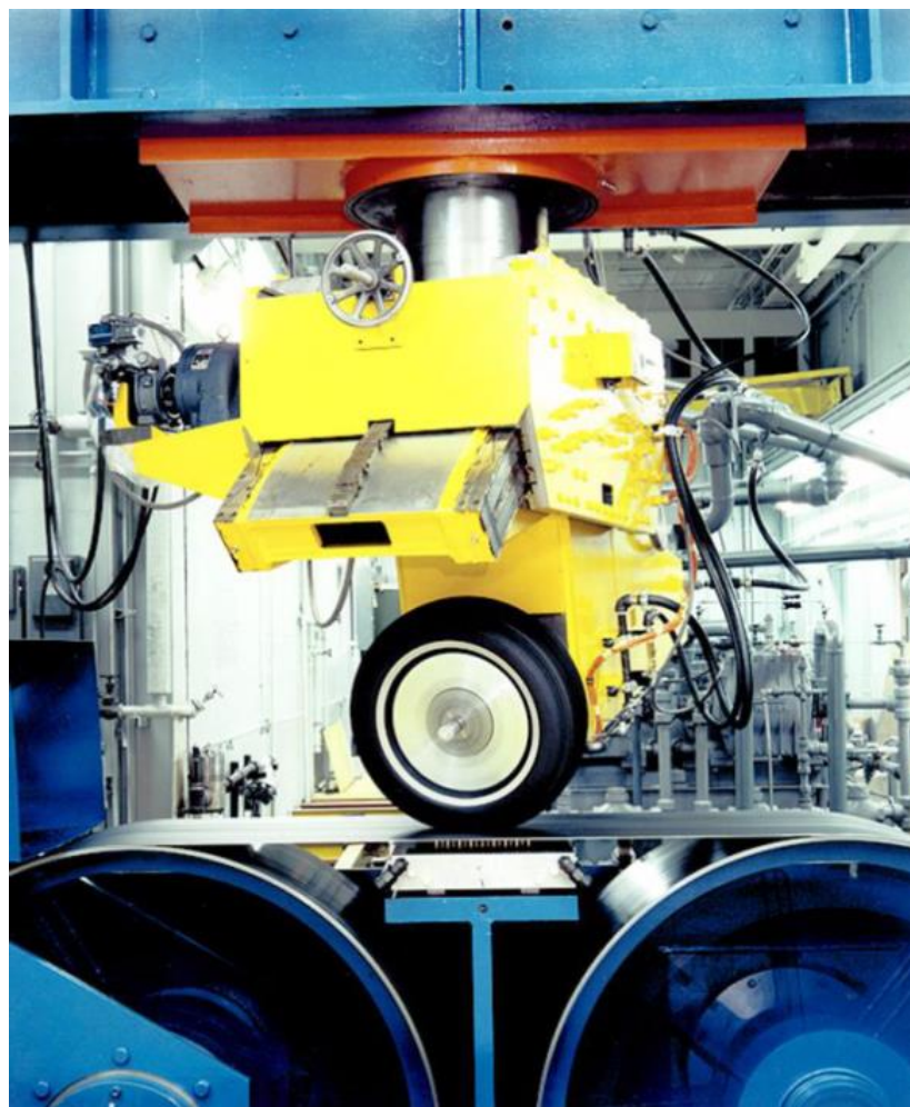
Figure 2.4 The flat trac tire test rig at Calspan's Tire Research Facility [34]
