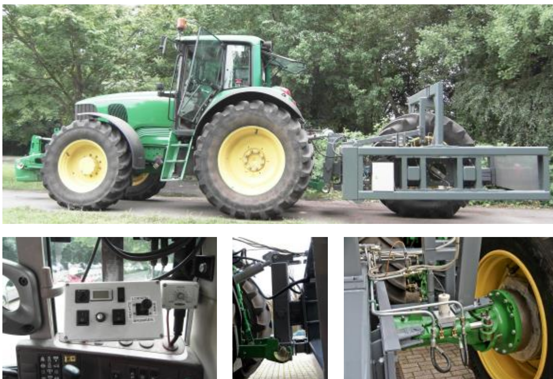
Figure 4.7 The photo of the tractor and mobile tire test rig - top, the Joystick – bottom left; the gap between the ‘tractor’ and ‘front’ section- bottom middle; the wheel suspension – bottom right
