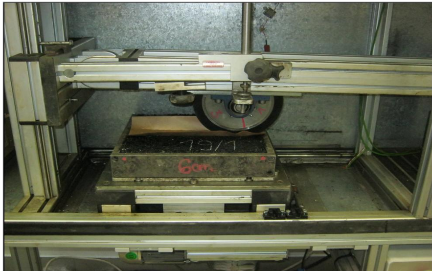
Fig.5.34: Schematic view of the laboratory wheel track test
