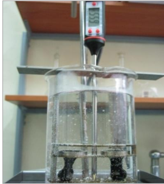
Fig. 5.13: Softening point test
