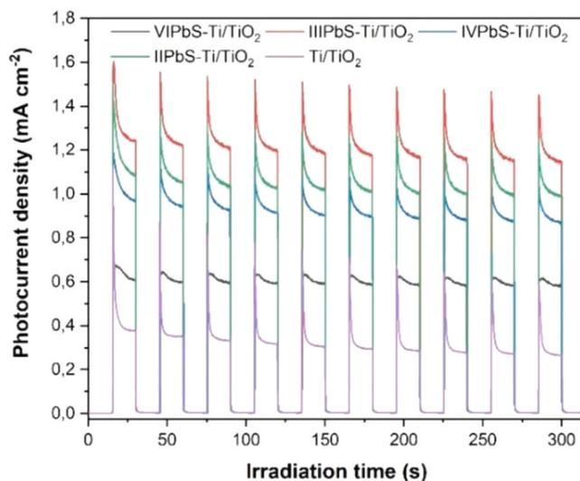
**Fig. 5.** Photocurrent response at +1 V/Ag=AgCl of Ti/TiO<sub>2</sub> and PbS-Ti/TiO<sub>2</sub> photoelectrodes.
