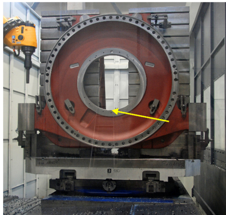
Figure 1. View of a large-size workpiece mounted on the table of the WHN 13-15 CNC machine. The roughness measurement point is indicated.
