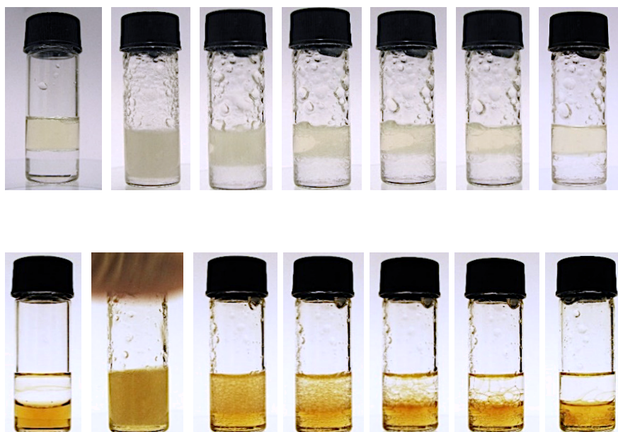
Figure 27. A) Demonstration of the phase separation between the upper aqueous phase containing Ac-IONPs and lower chloroform phase. Images from left to right shows the rapid phase separation after vigorous shaking, B) Demonstration of the phase separation between the lower chloroform phase containing OA-IONPs and upper aqueous phase. Images from left to right shows the rapid phase separation after vigorous shaking.
