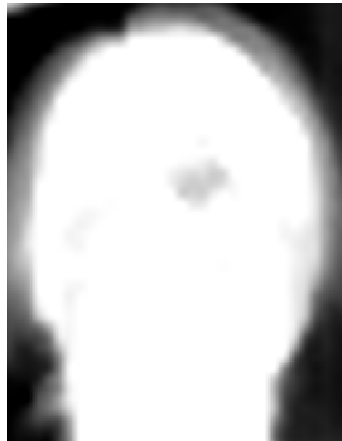
Figure 4.3. Thermal image of a face (cropped to a facial area) scaled from a full raw data range to a full output image range resulting in a complete loss of facial features visibility
