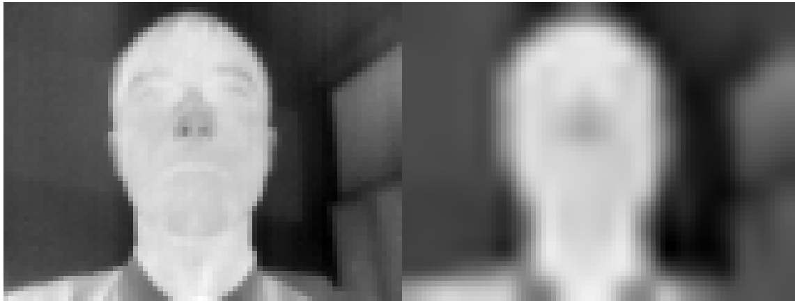
Figure 5.1. Example of thermal image of a face (on the left) and its corresponding LR version generated by downscaling and then upscaling of an original image by a factor of 4
