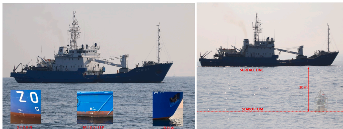
Fig. 3. Draught of tested vessel during measurements (left) and UMM sea bottom placement (right).
