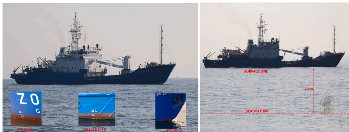
Fig. 3. Draught of tested vessel during measurements (left) and UMM sea bottom placement (right).
