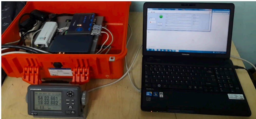
Fig. 9. Real-time satellite navigation data recording system.
