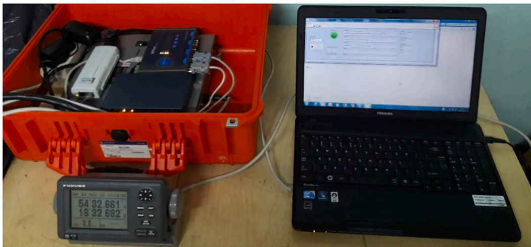
Fig. 9. Real-time satellite navigation data recording system.
