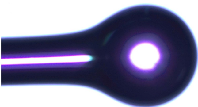
Figure 2. A microscope image of the microstructure used for supercapacitor in situ temperature measurement.
