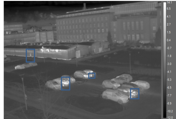
Fig. 3: Experiment 4 set-up. The thermogram with indicated heat sources like: cars engine, car tires and people
