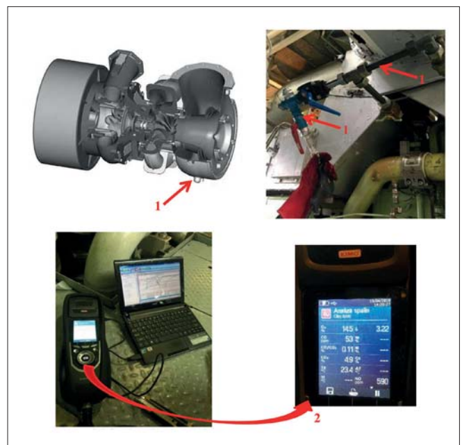
Fig. 10. Method of introducing the measuring probe of the exhaust analyser into the turbine exhaust duct of the turbocharger in the tested engine (a) and the view of the measurement set during the test realisation (b): 1 - drainage channel [21], 2 - magnification
