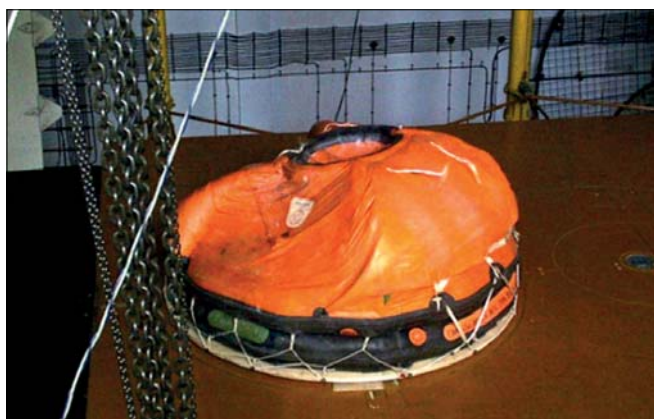
Fig. 4. Life raft during wind tunnel teste (research report, 2000)
